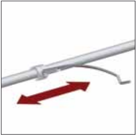
Coulissage des composants le long du profilé Components can be slid along the profile rail
